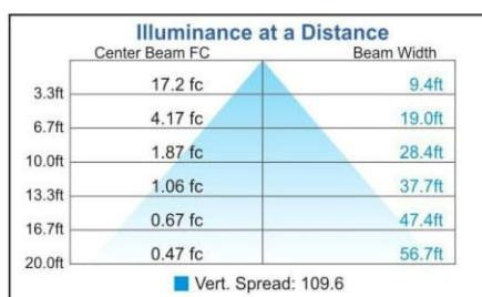
Note: The Curves indicate the illuminated area and the average illumination at a set distance from the LED Down Light.
