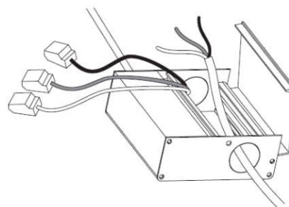
6. Place all wiring and connections back in to the box and close the cover. Connect the driver to the light panel.
